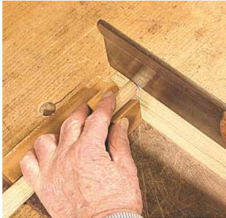
▲ Pic. 5 Saw a very shallow kerf to form the shoulder line
